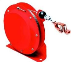
Static Bonding Reels provide the automatic retraction and compact storage of 50, 75, and 100 foot cable and clamp assemblies. Designed to function under extreme environmental conditions, the 50 and 75 foot cable length models meet USAF specification MIL-
