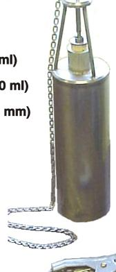
The unique Model GTP-9021 was developed specifically to fit through the small gauging found on U.S. Air Force bases where level gauging electric cables are also present. It was important that there be no tangling of our sampler with those cables and that the cables not be damaged. Therefore, the outside diameter is only 3.1 in. (79 mm)
